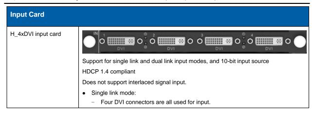
Each connector supports the maximum resolution of 2048x1152@60Hz and the minimum resolution of 800x600@60Hz.
